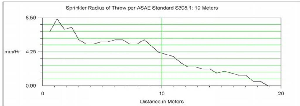
The "Single-Leg Diagram" shows the distribution of water thrown from a nozzle (mm/hr) versus the distance from the nozzle (0 to 20 m in this case). Manufacturer's produce their own data (in .prf files) but it is best that is validated by an independent testing facility (such as at the Center for Irrigation Technology).
